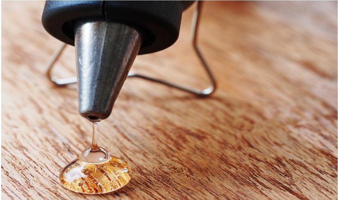
Figure 11 adhesives solidify by cooling
